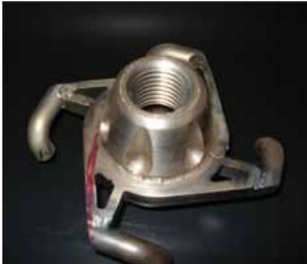
The original component was a fabrication of seven separate pieces welded together.
