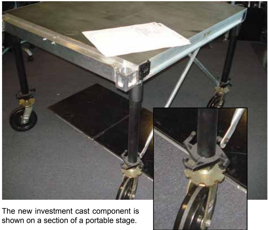
The new investment cast component is shown on a section of a portable stage.
